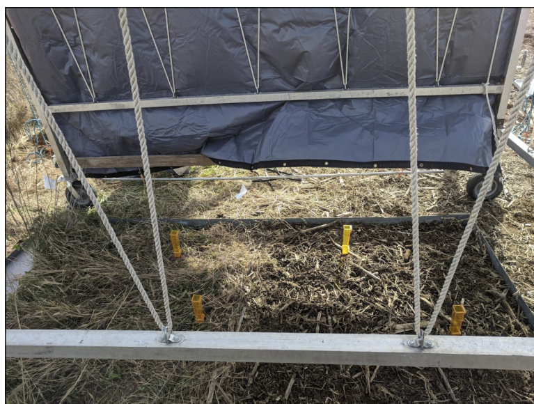
A view of the sampling set up under a rainfall simulation.
