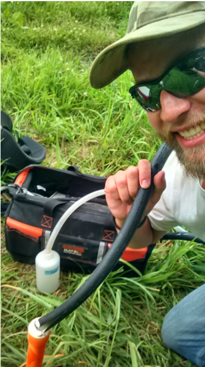
Pumping the solution of isotopically labeled nitrate into a piezometer using a peristaltic pump.
