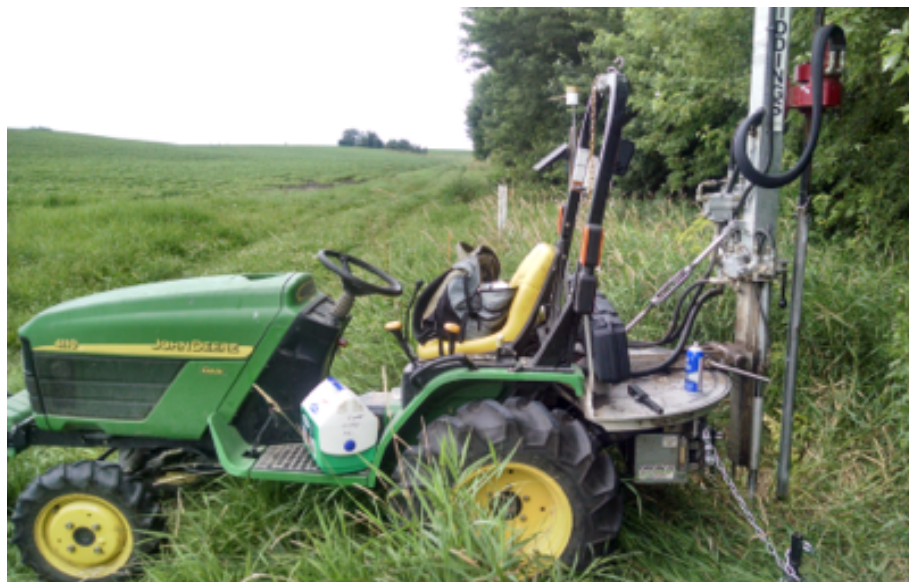
Hydraulic soil probe mounted to a tractor. This unit is used to collect the 3.28 feet deep cores in order to measure denitrification.
