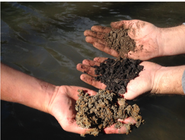
Walnut Creek streambanks are composed of three very different soils, stacked horizontally like a giant layer cake. A key objective of the study is to determine the erosion rate of each layer. (Photo by Hanna McBrearty)
