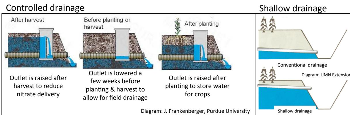
Figure 1. Generalized diagram showing general processes involved with both controlled drainage and shallow drainage practices. Controlled drainage diagram (left hand side): J. Frankenberger, Purdue University, 2014; Shallow drainage diagram (right hand side): Bushman and Sands, 2012.
